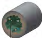
Lack of corrosion control allows lead to leach from pipes into water.
